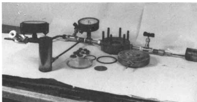
Fig. 1. Reverse osmosis unit fabricated in NCL.
